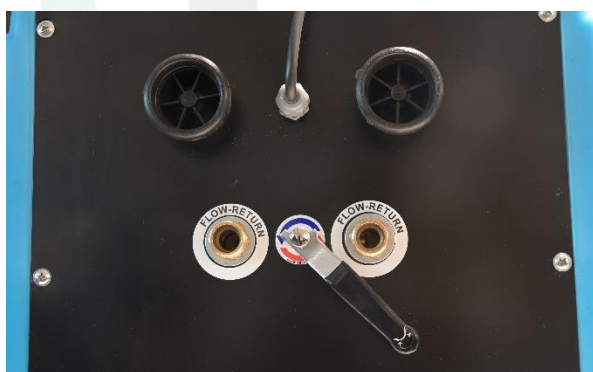
PUMP FLOW TO THE RIGHT, RETURN TO THE LEFT
